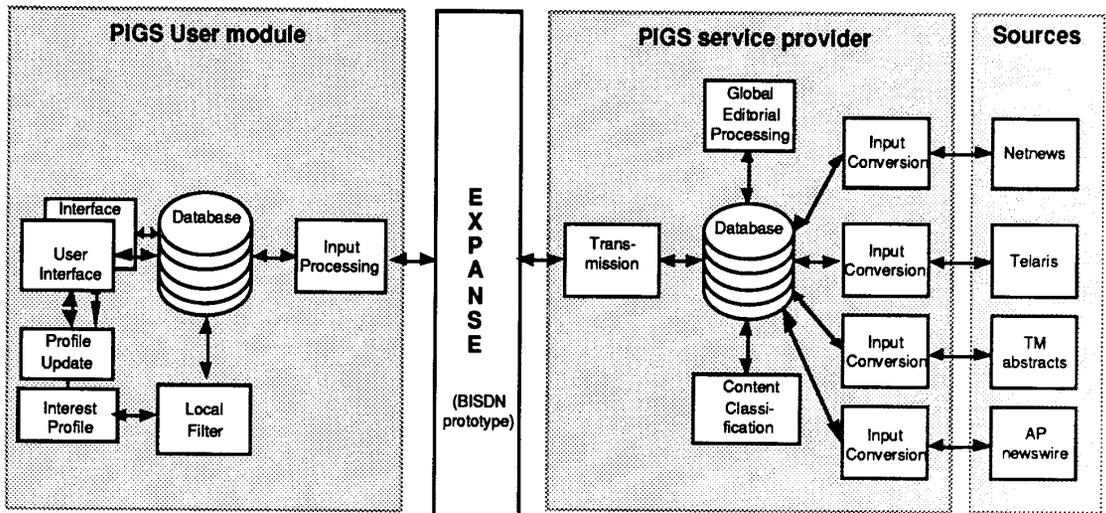
Figure 1. PIGS prototype software architecture
